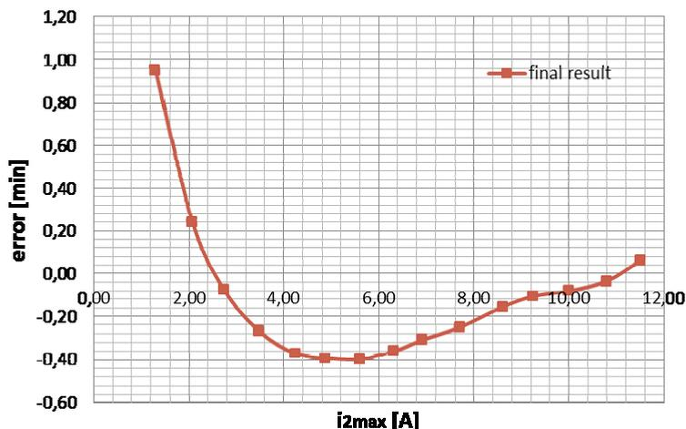
Fig. 6. Double-core current transformer's error final result
