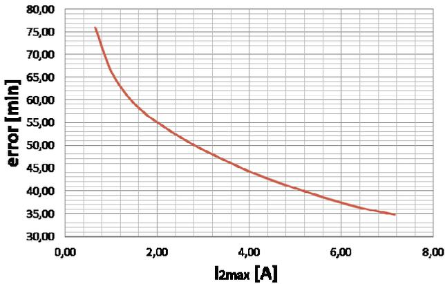
Fig. 4. Current transformer error with no compensation
