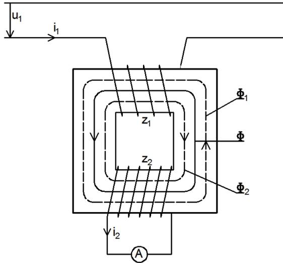
Fig. 1. Streams induced in the magnetic circuit transformer [1]
