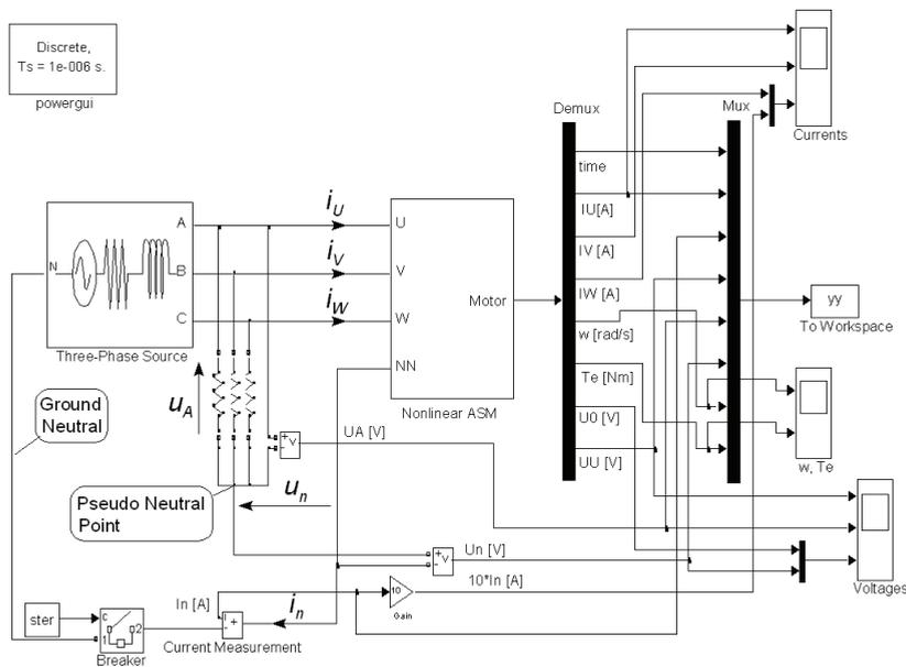
Fig. 2. The main system connecting the saturating induction machine with the external circuit (here: Three-Phase Source) in Simulink
