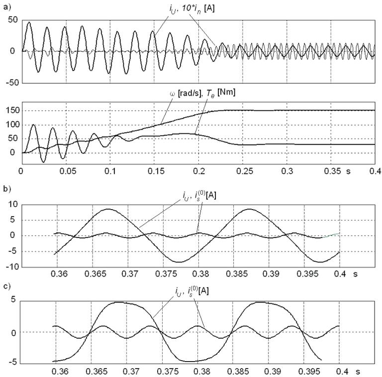
Fig. 4. Free acceleration starting of loaded induction motor (a) (connection: in star with the ground neutral) and steady state waveforms of phase current and the stator current zero symmetrical component: b) for loaded motor, c) for unloaded motor
