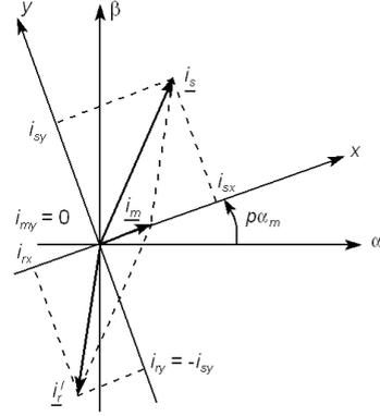
Fig. 1. Illustration for transformation from the stationary reference frame  $\alpha$ - $\beta$  to the magnetising current oriented  $x$ - $y$
