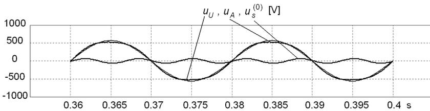
Fig. 5. Steady state waveforms of phase voltages (for the motor and the mains) and the zero voltage symmetrical component
