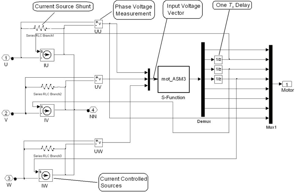
Fig. 3. Simulink model of a non-linear induction machine with the set of differential equations **mot\_ASM3** establishing S-Function
