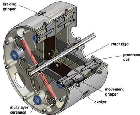
Fig. 3. Structure of the completed hybrid piezoelectric motor [6]
