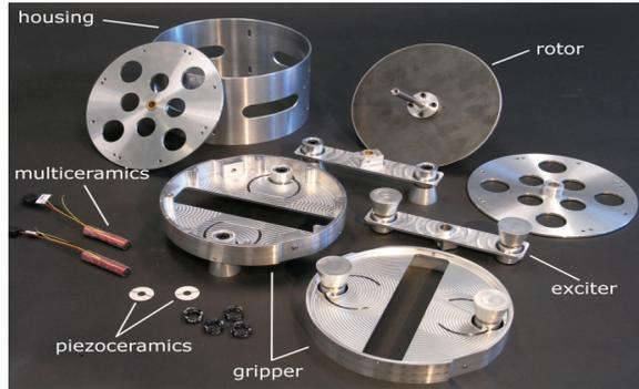
Fig. 5. Disassembled hybrid piezoelectric [6]
