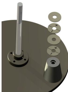
Fig. 4. Orientation of the ceramics and the electrodes
